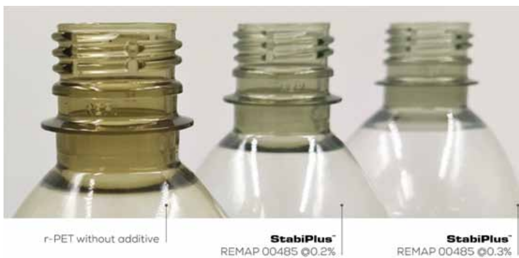
Picture 1: Bottles of 100% r-PET from mechanical recycling containing StabiPlus™. Being a liquid formulation, concentration is very high and related dosages minimal.
