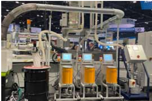
Picture 3: REPI's dosing units contain the basic colours necessary to obtain the target blue shade.
