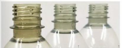
rPET brightness and shade improve cycle after cycle. Each of the three cycles has been designed to put maximum stress on the material in order to show the additive's performance: one lab cycle delivering double the stress of an industrial process. StabiPlus has been added to the first recycling loop only.
