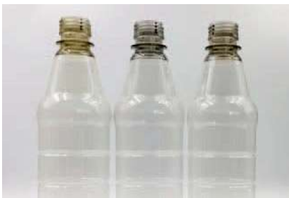
F.I.t.r.: 100% rPET, 100%rPET with AY 00015 @0.03% and same with AY 00201 with optical brightener @0.03%
