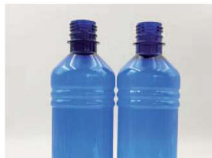
A dark blue on virgin PET (left) and on 100% rPET (right)
