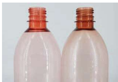
Antique rose with virgin PET (left) and with 50% rPET (right)
