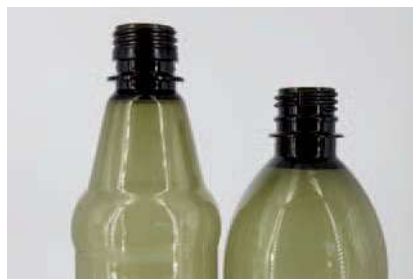
Olive green with virgin PET (left) and with 50% rPET (right)
